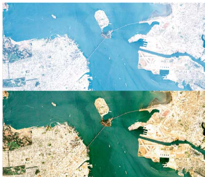
Fig. 2. Example of LEDAPS atmospheric correction. (a) Top-of-atmosphere (TOA) reflectance composite (bands 3,2,1) for Landsat-7 ETM+ image of San Francisco Bay (July 7, 1999); (b) Surface reflectance composite. Both images are linearly scaled from \rho = 0.0 to 0.15.
