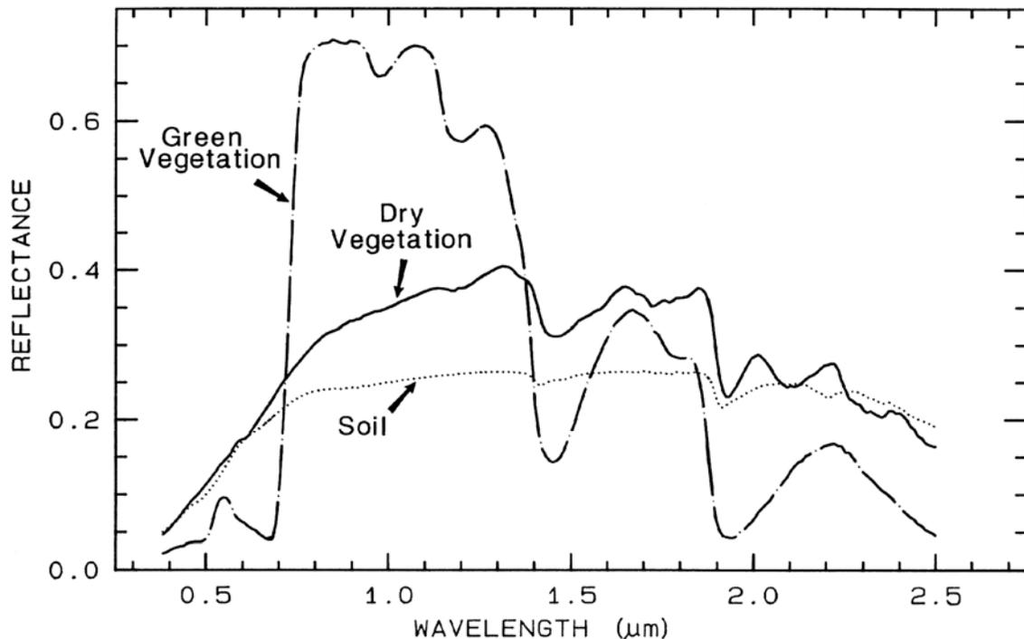
Very precise measurements can be made of the reflectivity of materials that more easily reveal their subtle differences. Above is a plot of the reflectivities of green vegetation, dry vegetation and soil between wavelengths of 0.4 and 2.5 micrometers. Scientists use graphs such as these to design instruments that help them discriminate between a variety of interesting materials and mineral deposits.
