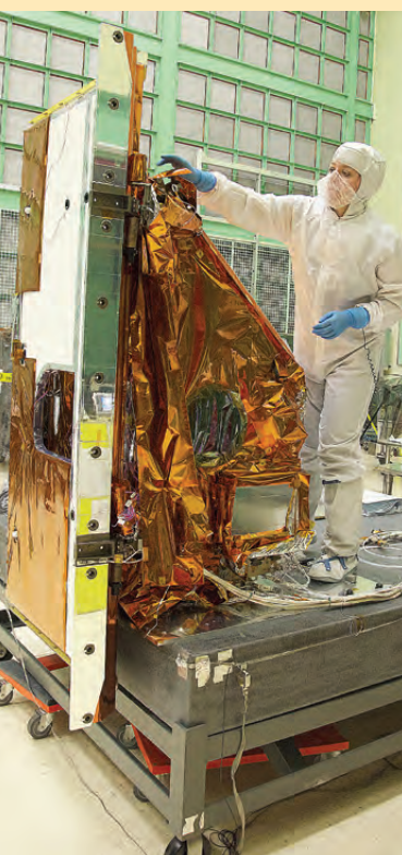
A technician reaches across the instrument to affix the corners of a multi-layer insulation blanket to the TIRS instrument.
