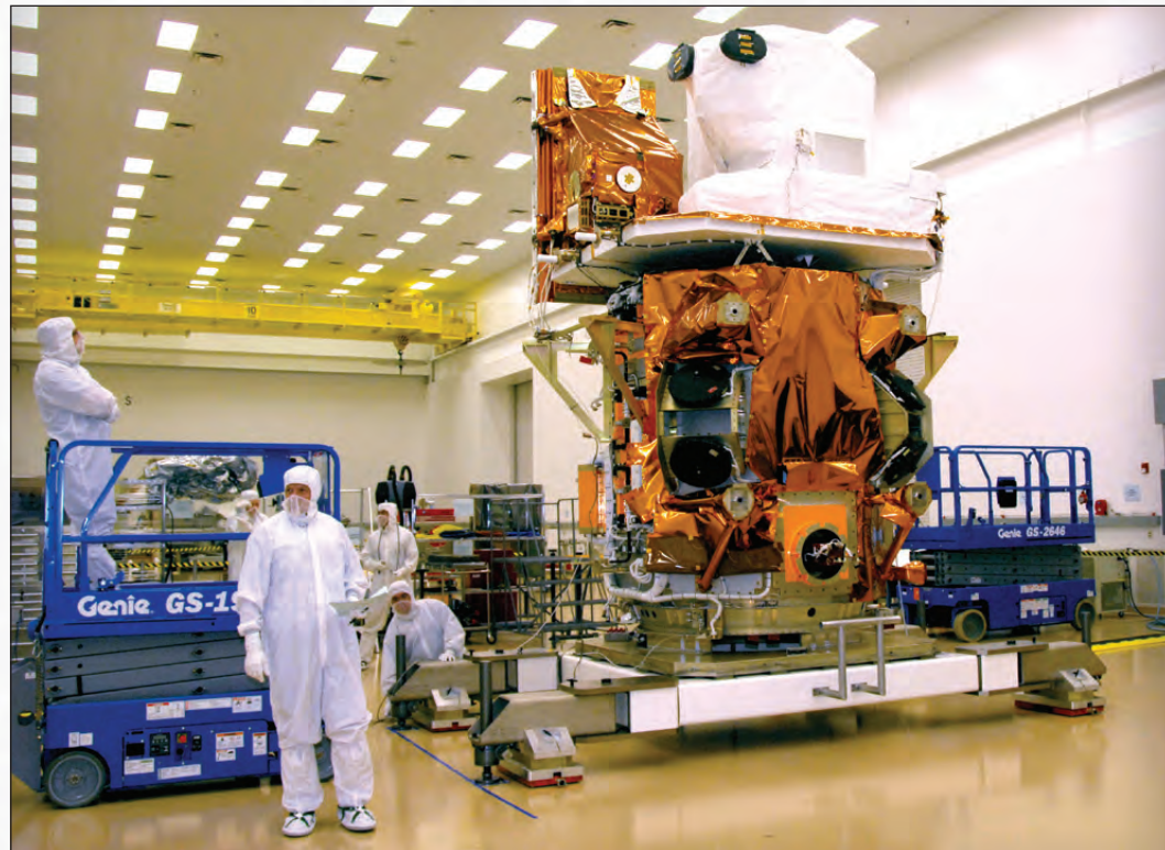
The LDCM observatory consists of the spacecraft bus with the instruments mounted on top in this photo..
